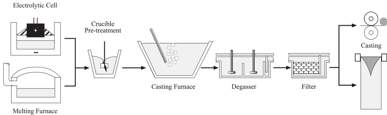
Figure 1: Sequence of Molten Metal Processing Steps.
