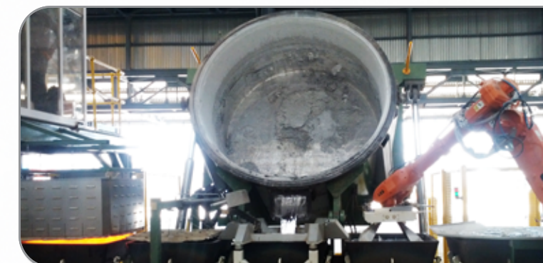
Hydraulically-operated crucible tilters directly into the sow moulds
