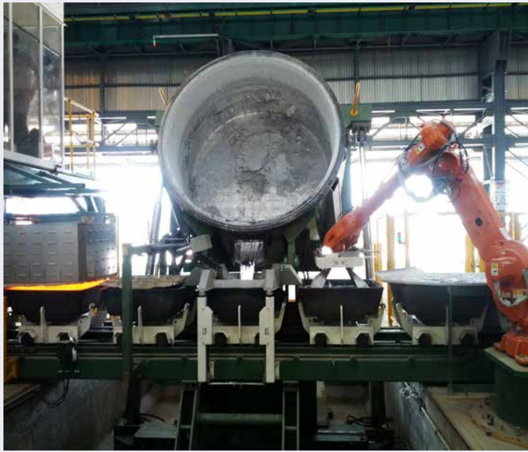
Hydraulically-operated crucible tilters directly into the sow moulds
