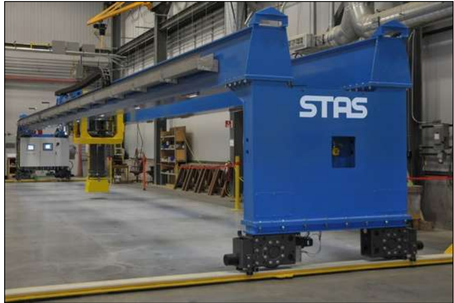
Figure 1. STAS pot ramming machine.
