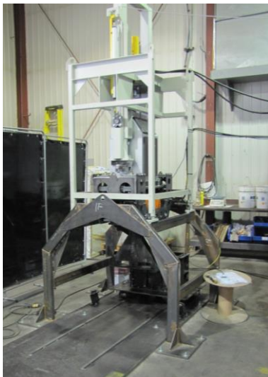
Figure 1. Full scale compaction bench test.
