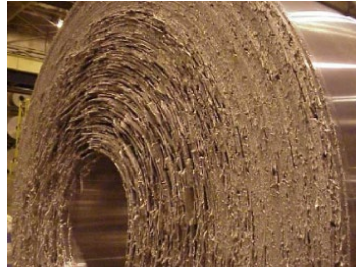
AA5182 edge cracking caused by excess Na during hot rolling and after coiling
