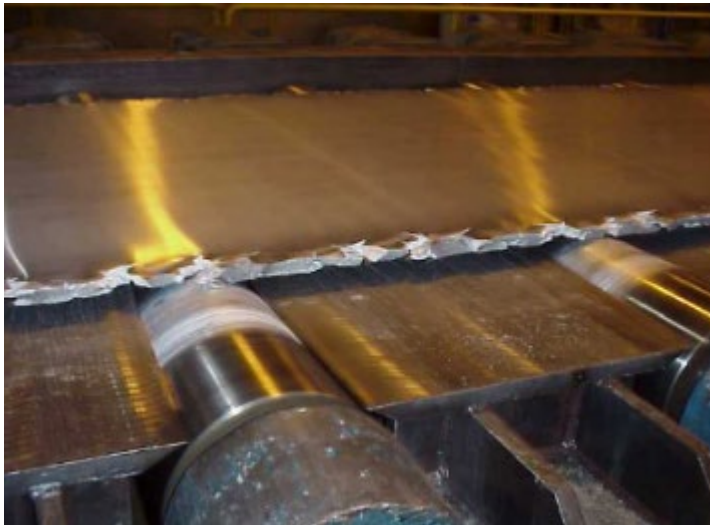
AA5182 edge cracking caused by excess Na during hot rolling and after coiling
