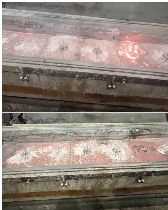
Figure 7. Monitoring of AA3104 aluminum using chlorine (top) and AluCLEAN (bottom).
