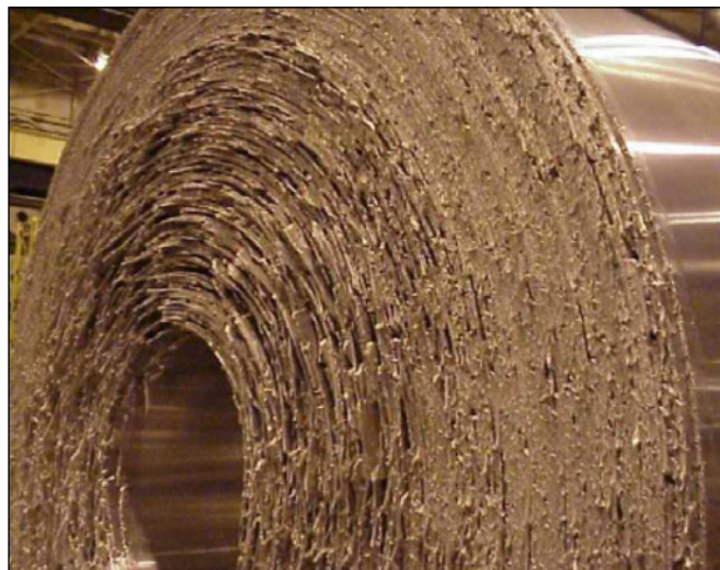
Figure 1. Edge cracking of AA5182 caused by excess Na after coiling. 1
