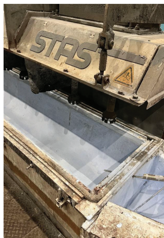
Pic 2. AluCLEAR rod injection point
